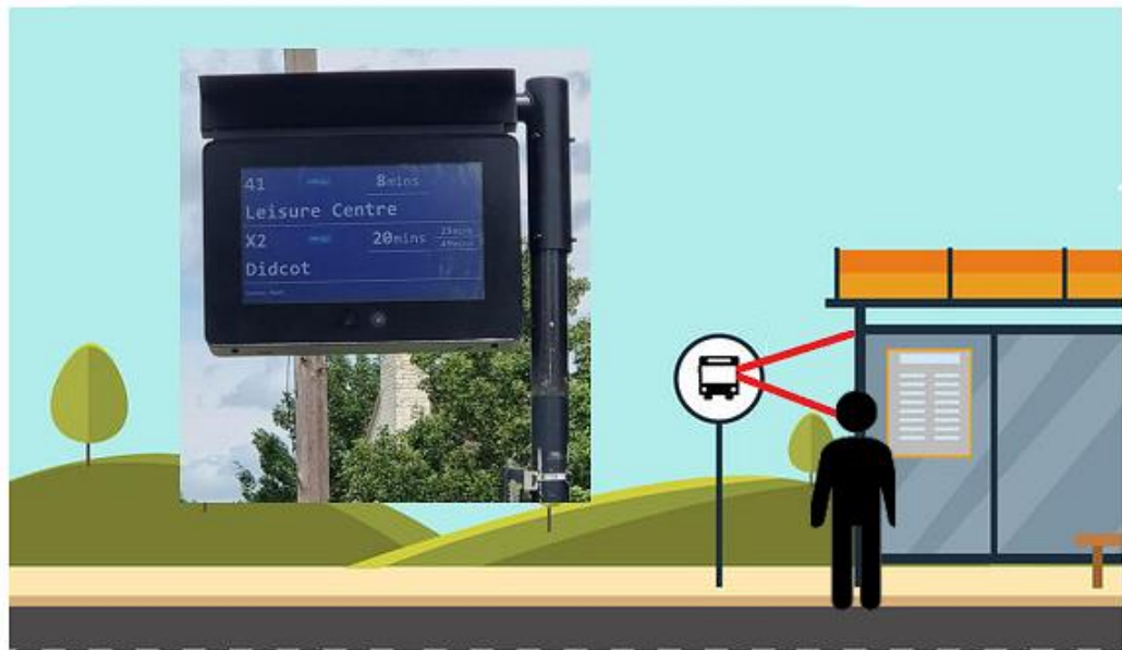
Figure 4 A TFT display installed on a low pole to reduce reflections © M2M Tech
